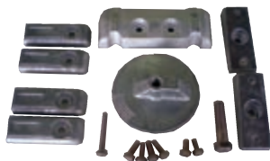
TEC 20816 Mercury Verado 6-Cyl Engine Kit Zinc
