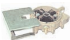
(1) Depress Brushes and Slide End Cap In Tool
