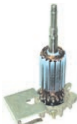
(3) Remove Tool Leaving Brushes Loaded For Assembly
