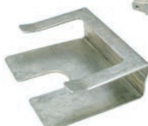
(3) Remove Tool Leaving Brushes Loaded For Assembly
